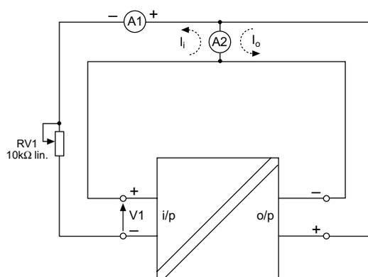
Ammeter A2 must be capable of handling either polarity of signal. If it is not an auto-ranging instrument, set it to a high range before switch on, then adjust sensitivity to obtain the required reading.
