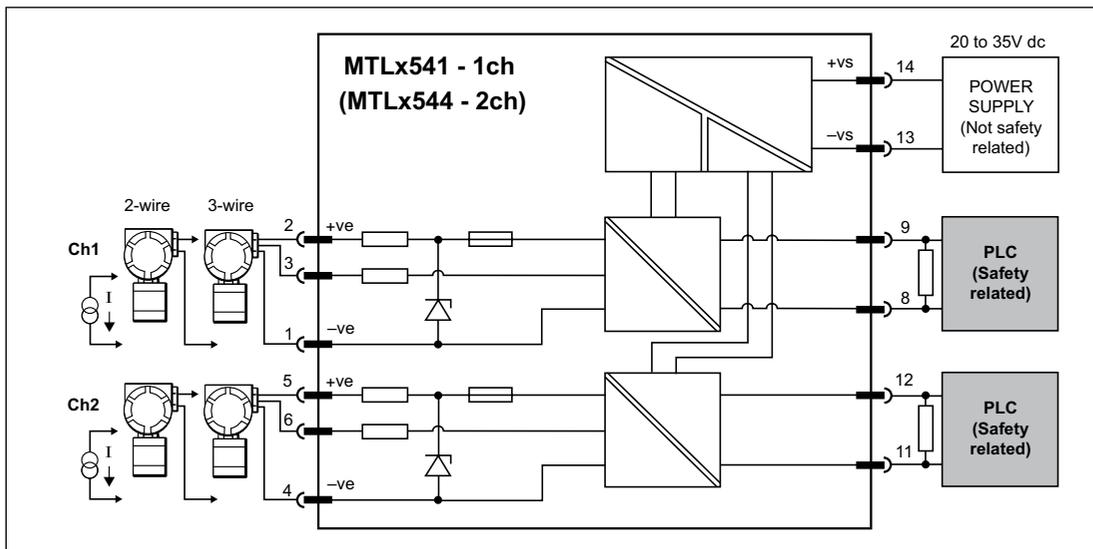
Figure 2.1 - Analogue Input module system configuration - see the "Note" in the text regarding use of dual channel modules.
