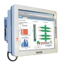
Azonix is introducing the Barracuda BOP, an application specific rig floor computer with integrated features required in blowout preventer surface systems. This workstation has a 19 inch LCD large enough to display clearly in one screen, all the critical information such as the complete Christmas tree, thereby avoiding the need to toggle between multiple screens. The unit has a hardware button that enables and disables the touch screen avoiding unsolicited touches that can impact the process.
