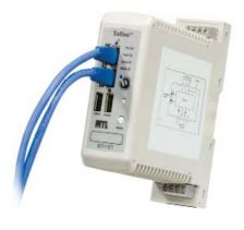
Tofino Security Appliance (SA) Creates Plug-n-Protect zones of security for SCADA networks
