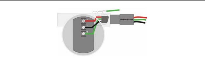
Figure 2 Connection detail for a typical process transmitter
