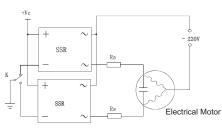
The time between the positive and negative rotation must be bigger than 20ms.
