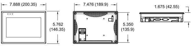
VESA Mount: VESA 75 (75 mm x 75 mm). Use four screws (M4-0.7 mm) less than 8 mm long.
